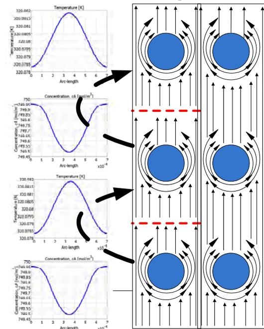
**Figure 2.** The visualization of the implemented pellet structure same, and these pellets were taken into one domain, which domain's size was equal the aggregated domains of the built bed. The pellet by pellet model was compared to this model. The pellet by pellet model is working as a network of pellet models. The output parameter profiles of the first pellet models are the second pellets inlet
