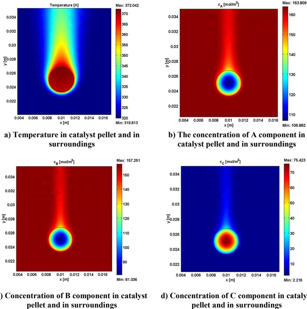
**Fig. 3:** Changes in the value of state-variables along the investigated part of reactor in steady-state
