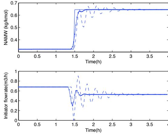
Figure 2. – Comparison of the grade transitions with initial parameters (dashed line) and with the experimentally determined parameters (dotted line)
