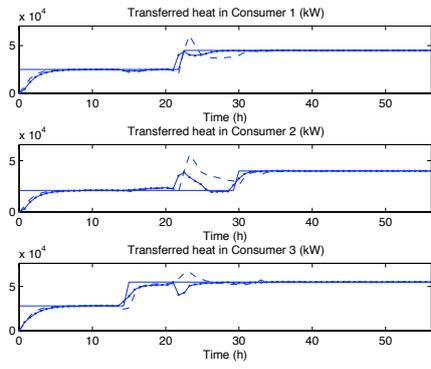
Figure 6: Comparison of the transitions in outputs with initial parameters (dashed line) and with the experimentally determined parameters (dotted line)
