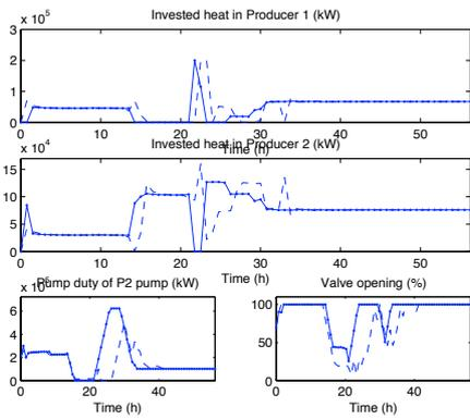
Figure 7: Comparison of the transitions in inputs with initial parameters (dashed line) and with the experimentally determined parameters (dotted line)
