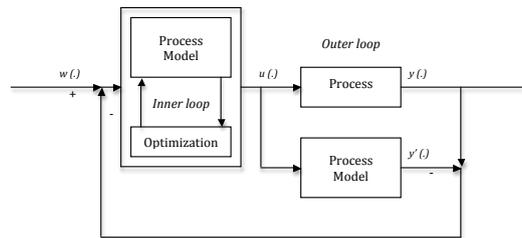
Figure 4: The scheme of the implemented non-linear model predictive controller
