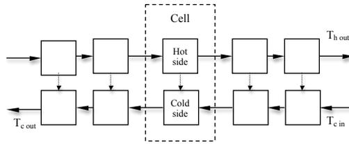
Figure 2: Cell model of the heat exchanger
