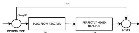
**Figure 3 The structure and the model parameters**
